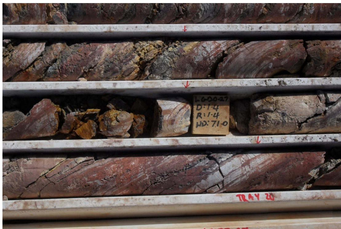
Figure 69. Example of drill core (LGDD_027) showing poor competency and cavities. Hole depth 71m.
