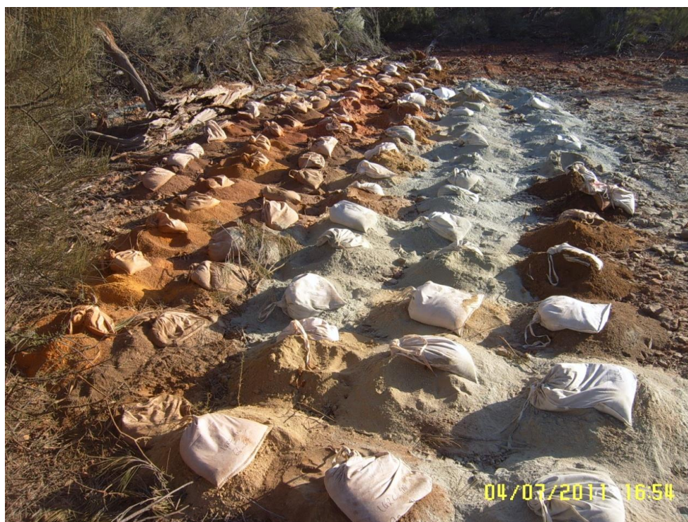
Figure 19. Drill samples laid out prior to collection and dispatch to assay laboratory.
