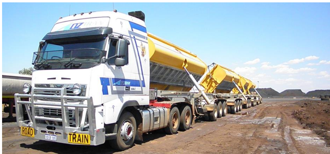
Figure 81. Typical Quad Side Tipper Road Train
