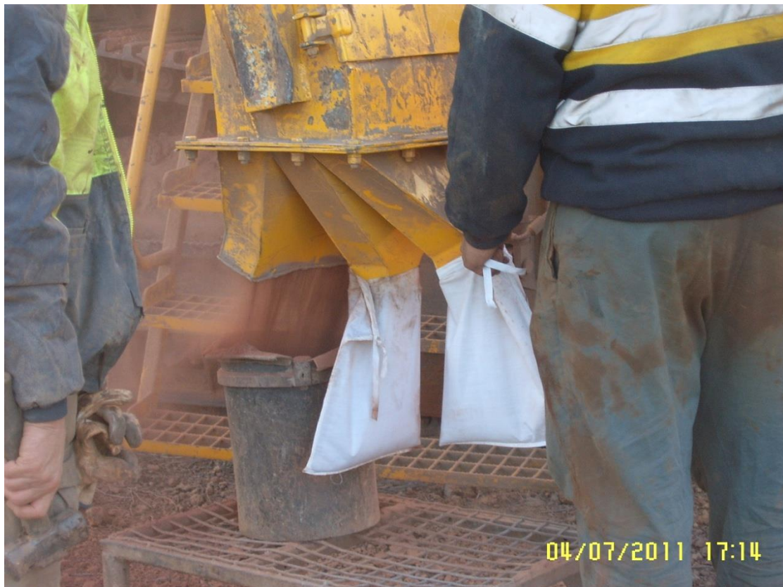
Figure 37. Three tiered splitter on RC drill rig, showing collection of primary sample and field duplicate. Sample residue collected in bucket.
