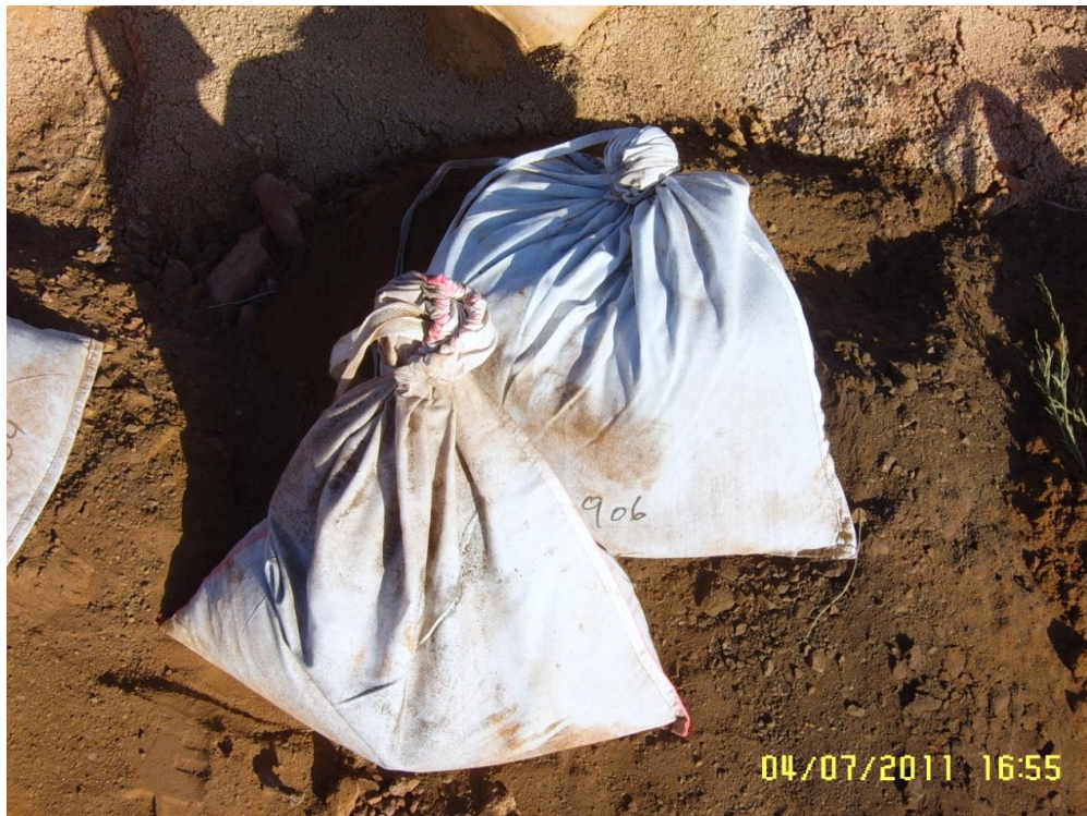
Figure 38. Primary sample and field duplicate laid out on sample piles on ground.
