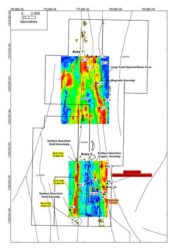
Figure 1. Hillside SkyTEM survey flown at 150 m line spacing showing conductors and geochemical anomalies.
