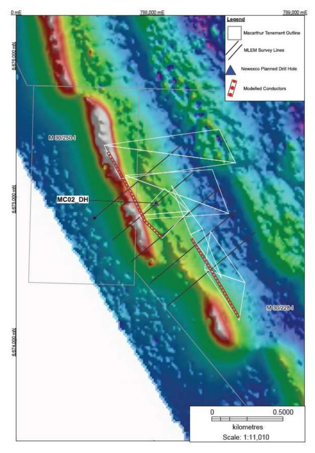
Figure 1. MLEM survey at Moonshine showing modelled conductors. Background image shows magnetic anomalies.
