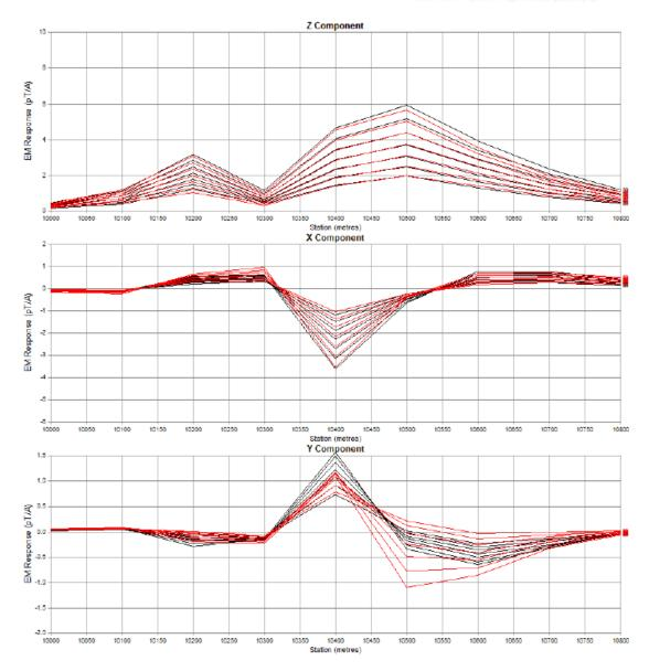
Figure 3. Late time (Ch33-Ch39, 101ms - 371ms) Linear profile at Moonshine MLEM line 50800N. Both showing modelled response in red versus field data in black. Very strong bulge characteristics of Bedrock Conductors.
