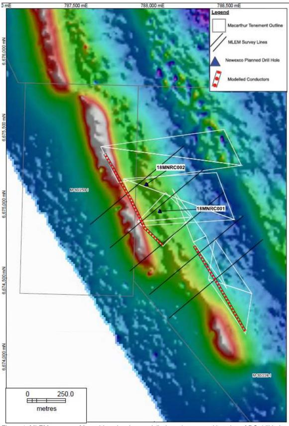
Figure 1. MLEM survey at Moonshine showing modelled conductors and location of RC drill holes. Background image shows magnetic anomalies.
