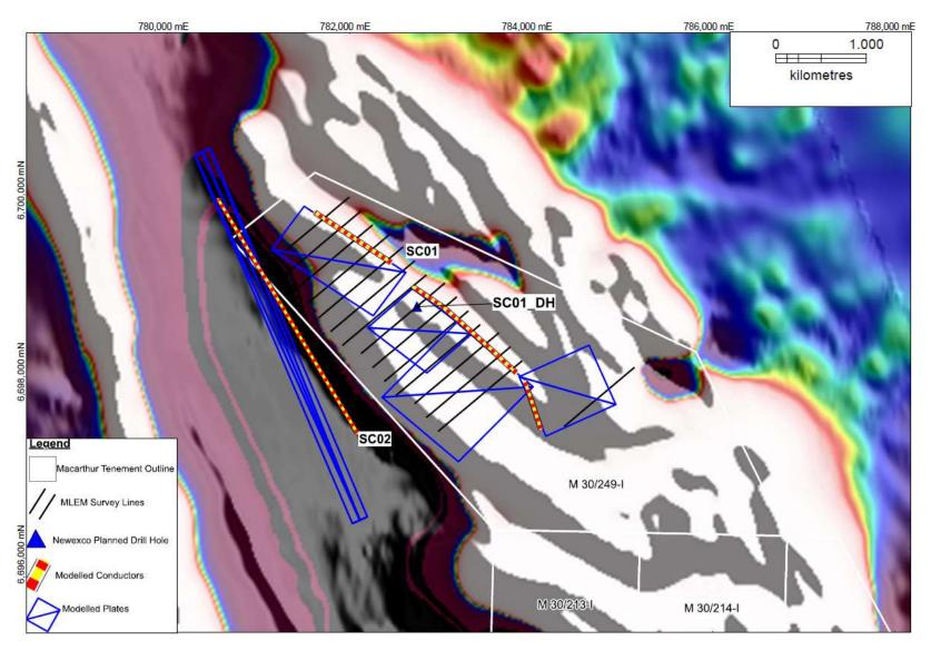
Figure 2. MLEM Survey at Snark showing modelled conductors. Background shows Total Magnetic Intensity anomalies
