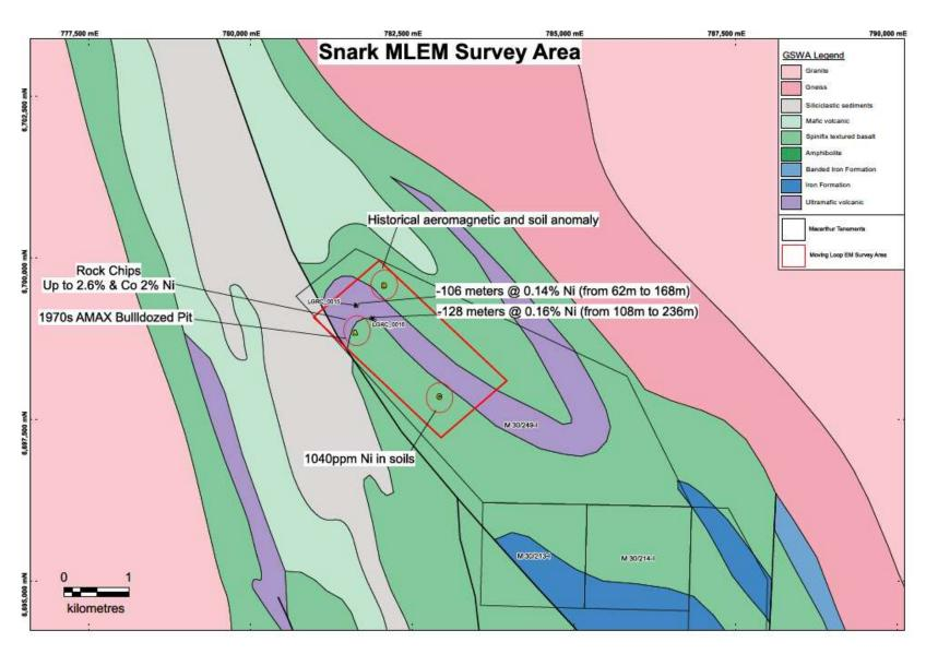
Figure 1. Macarthur's Lake Giles Moving Loop EM survey target area at Snark. Map shows the various Nickel and Cobalt anomalies at surface.
