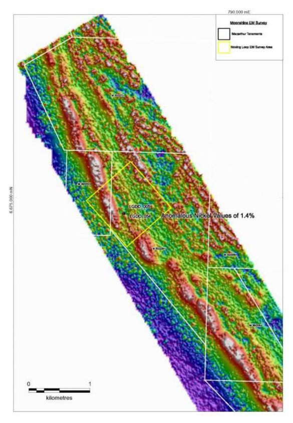
**Figure 2**. Macarthur's Lake Giles Moving Loop EM survey target area at Moonshine. Map containing 50m Ground mag conducted in 2006.
