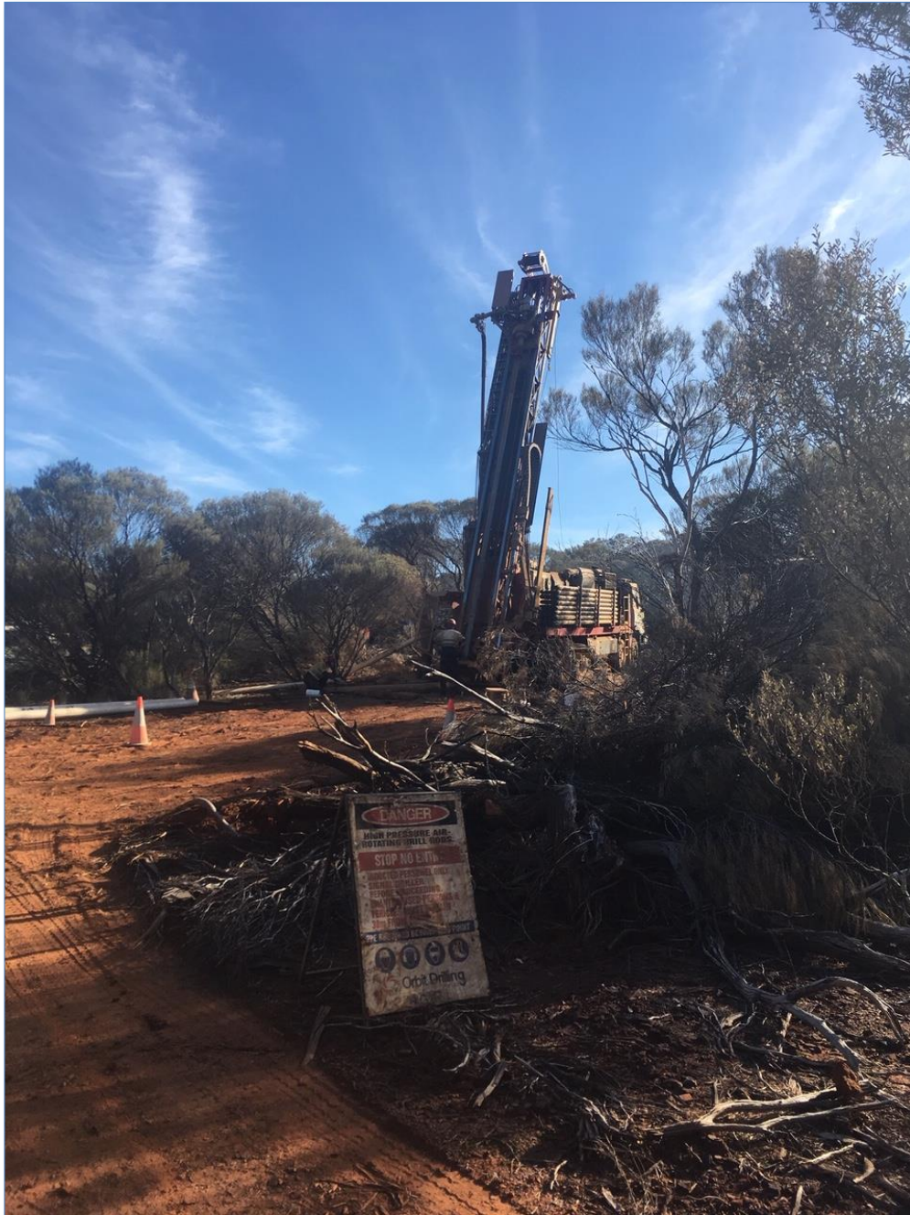
Photo 3 - Reverse Circulation Drill in action on hole LGRC2161 at Moonshine North.
