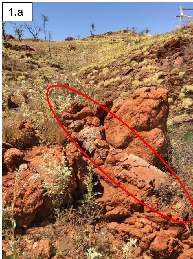
Figure 1. (a) Outcropping pegmatite in foreground showing lepidolite mineralisation at surface (circled); (b) Pegmatite sample dominated by lepidolite containing 1.47% Li 2 O.
